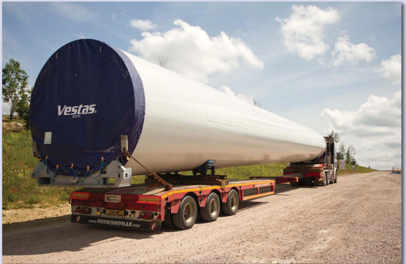
Tower section being transported to turbine location on site at Wadlow Wind Farm, Cambridgeshire. Photo courtesy of BIF.
